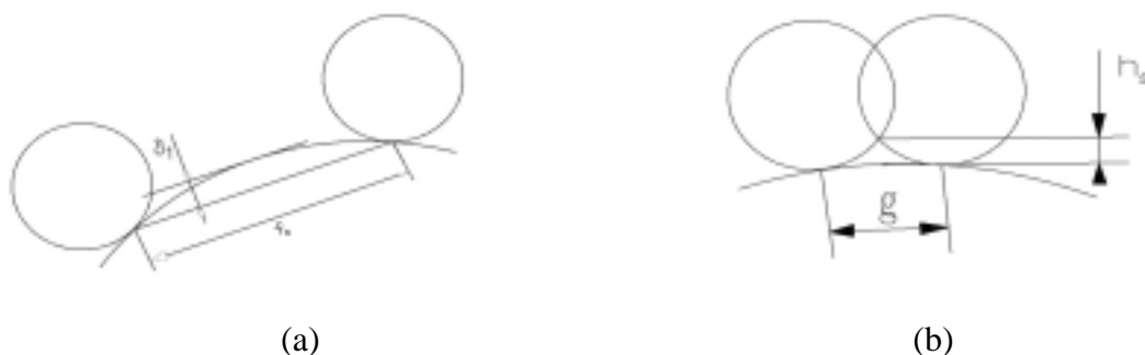
Figure 2. Forward step, cordal deviation (a) and scallop height resulting of two paths.
